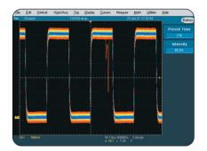
Elusive Glitch. Fast waveform capture rate, enabled by Tektronix proprietary DPX acquisition technology, maximizes the probability of capturing elusive glitches and other infrequent events.
