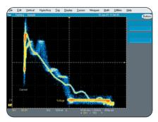
Display of a current vs. voltage trajectory XY plot of the DUT. This highly dynamic waveform display provides continuous coverage of device performance – the waveform data is continuously streamed to the display. Color-grading reveals the distribution of signal activity for comparison against device Safe Operating Area (SOA) characteristics.
